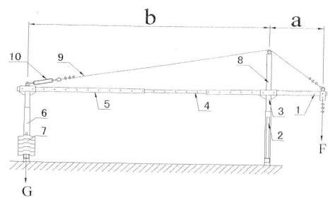
Figure 2: Suspension Mechanism
